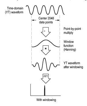
The Math FFT function includes three FFT Window options. There is a trade-off between frequency resolution and amplitude accuracy with each type of window. What you want to measure and your source signal characteristics will help you to determine which window to use.
