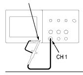
2. Set the switch to 10X on the P2220 probe and connect the probe to channel 1 on the oscilloscope. To do this, align the slot in the probe connector with the key on the CH 1 BNC, push to connect, and twist to the right to lock the probe in place.
