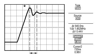
You can see the  $\Delta$  (delta) time and frequency (the measured ring frequency) in the Cursor Menu.
