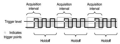
Triggers are not recognized during holdoff time.
