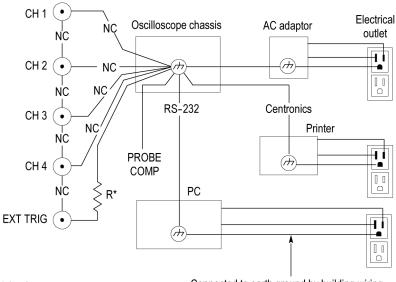
\* 3 MΩ impedance. NC means not connected.
