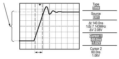
**NOTE**. The Rise Time measurement is available as an automatic measurement in the Measure Menu. (See page 102, Taking Measurements.)
